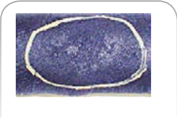
Hose with cover charred area from high heat or extreme aging due to heat or ozone
