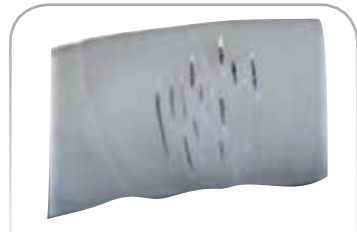
Hose with cover cracks due to age or the effects of ozone. Hose covers over time harden and should be replaced if this condition is found. (note: if boat has an ozone generator on board this could accelerate this condition
