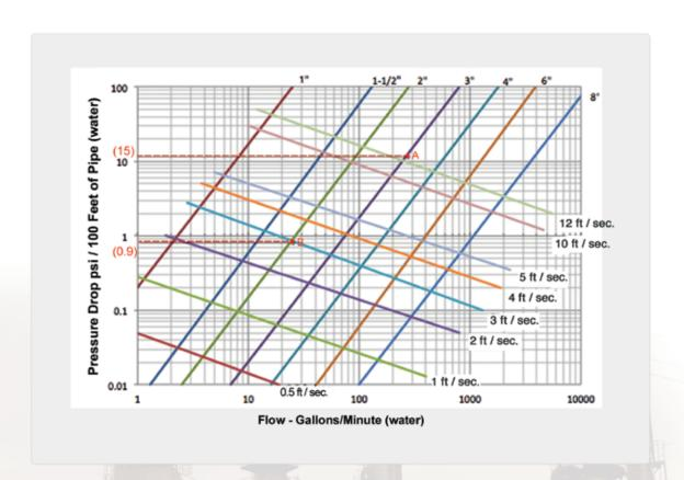
Pressure drop can be determined from head loss by applying the following formula:
