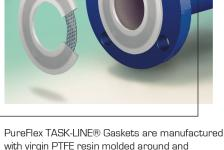
PureFlex TASK-LINE® Gaskets are manufactured with virgin PTFE resin molded around and through a stainless steel perforated metal insert. TASK-LINE Gaskets are recommended for chlorine service due to many advantages:
