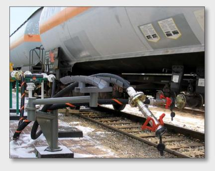
TODO-GAS® couplings are specifically designed for the safe transfer of LPG (typically Propane / Butane) in both liquid and vapour phases. The materials of construction and component design are specified to recognise the unique properties of LPG and terminal handling characteristics.
