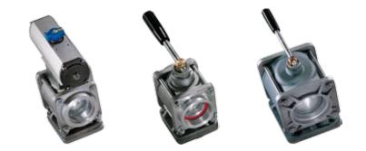
Similar in design to the one way valve, the two way performs a different function. Usually used as a compartment or tank switching valve, the two way valve has three ports — one inlet and two outlets. The valve directs the flow from the inlet to either of the two outlets. Features apply equally to both one way and two way designs. Available with a wide selection of end connections and actuation configurations.
