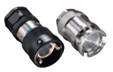
**1" Todo-Matic® (DN19 - DN32, Ø56 mm)** Todo-Matic® Dry Break® couplings in 1" size are designed for smaller bore applications where compact dimensions are required. One handed operation, high flow rate and minimal release on disconnection make Todo-Matic® perfect for transferring high value or sensitive medias with confidence. The addition of selectivity to prevent product cross contamination expands the operational possibilities in manifold exchange applications.
