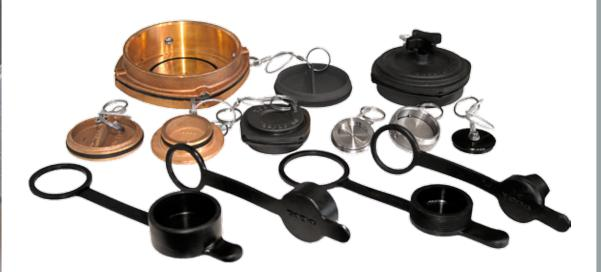
Available in stainless steel, brass / gun-metal and aluminium. There are also versions available in rubber. Dust plugs / caps should be used to prevent ingress of dirt or water. Sizes:  $\frac{3}{4}$ " - 6". Rubber only in 1" and 2".
